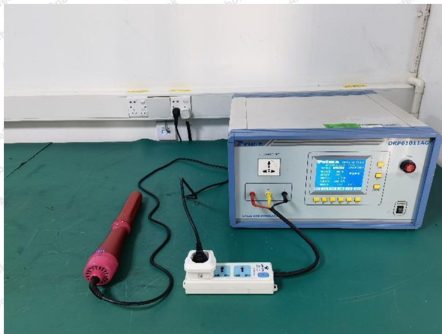
Photo of Voltage Dips and Interruptions Test
