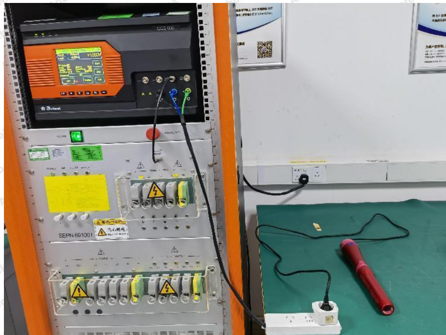
Photo of Surge Immunity Test
