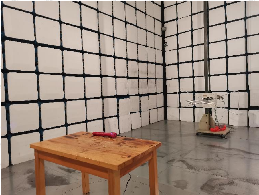
Photo of Radiated Emission Test
