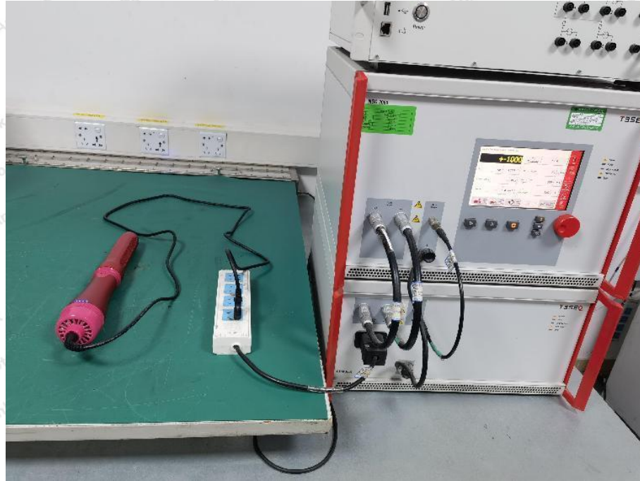
Photo of Electrical Fast Transient/Burst Immunity Test
