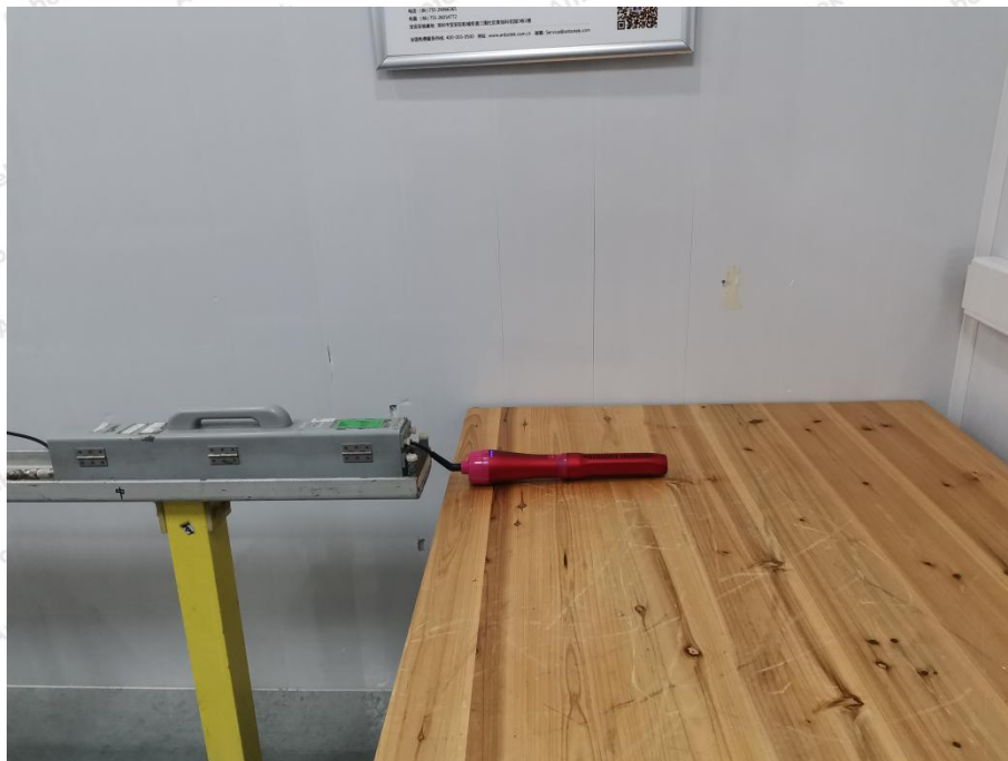
Photo of Disturbance Power Test
